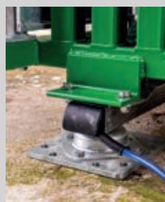
10 Integrated mounting plates for load bars HDST
