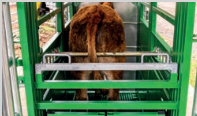
7 Animal restraint from the rear with rump bar
